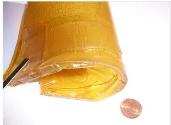
Fig. 1: Rubber slabs prior to comminution
