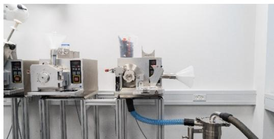
Fig. 3: PULVERISETTE 19 with high-performance Cyclone separator
