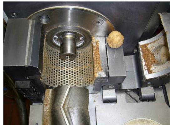
Fig. 4: The view into the opened grinding chamber shows an optimal throughput of the walnuts
