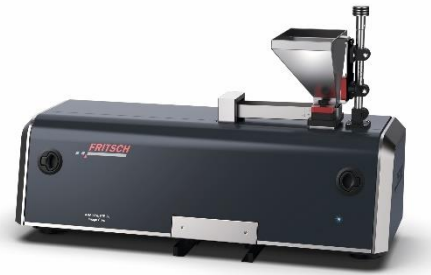
Fig. 3: ANALYSETTE 28 ImageSizer for dry measurement of particle shape and size of powders and bulk solids
