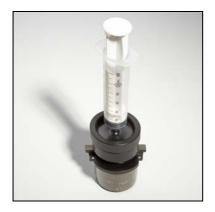
Tense the syringe firmly on the emptying device!
