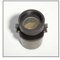
Firmly attach the emptying device with the sieve and seal ring onto the grinding bowl!
