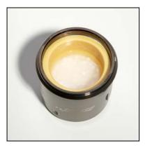
Bowl with balls and suspension after completion of the grinding!
